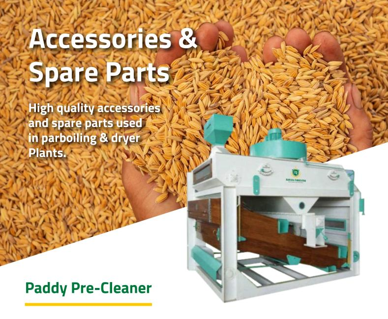
Paddy Pre-cleaner is used to remove extra-large impurities such as large stone, large soil clods, hemp rope and straw from raw paddy. This is done to optimize the storage life of the grain and to improve the quality of the product that has to be cleaned.
